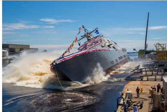
The U.S. Navy's future littoral combat ship USS Billings (LCS 15) launches sideways into the Menominee River in Marinette, Wisconsin,
